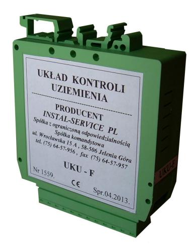
Control of ground continuity relay type UKU-F is designed to control the value of ground resistance of the receiver. The unit is designed for use in 3-phase grid with rated voltage of 400V, 500V, 1000V with insulated neutral point of the transformer. In the measuring circuit can be engaged contacts locks or other elements of the control circuit, thereby carring out the no voltage, remote control of external devices.
